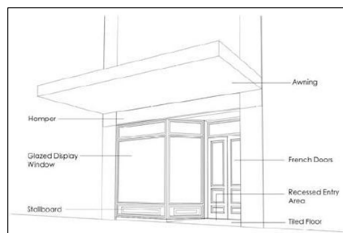
Figure 9.4-j: Elements of a traditional early twentieth century shop front (I)
